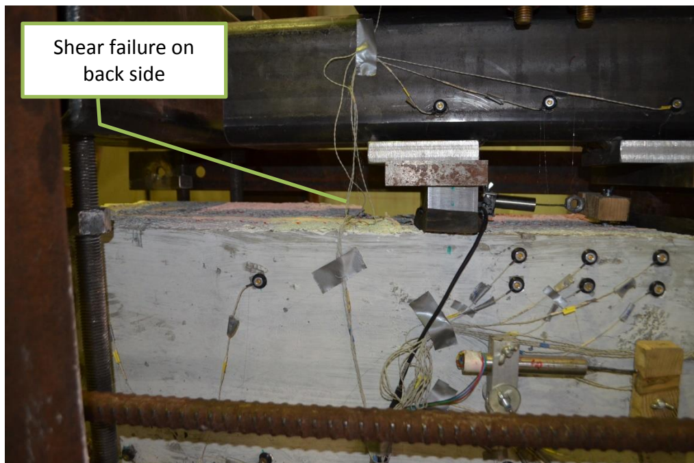
Figure 5-75: Specimen H1.25S1-M LED Side of Damaged Linear Moment Region after Failure
