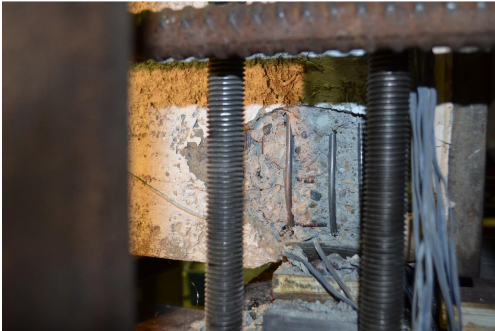
Figure 5-76: Specimen H1.25S2-C Support after Failure
