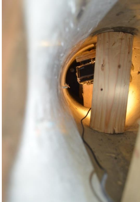
Figure 5-15: Specimen H1C2-C Wooden Braces Located at Load Points and Support to Avoid Punching Failure
