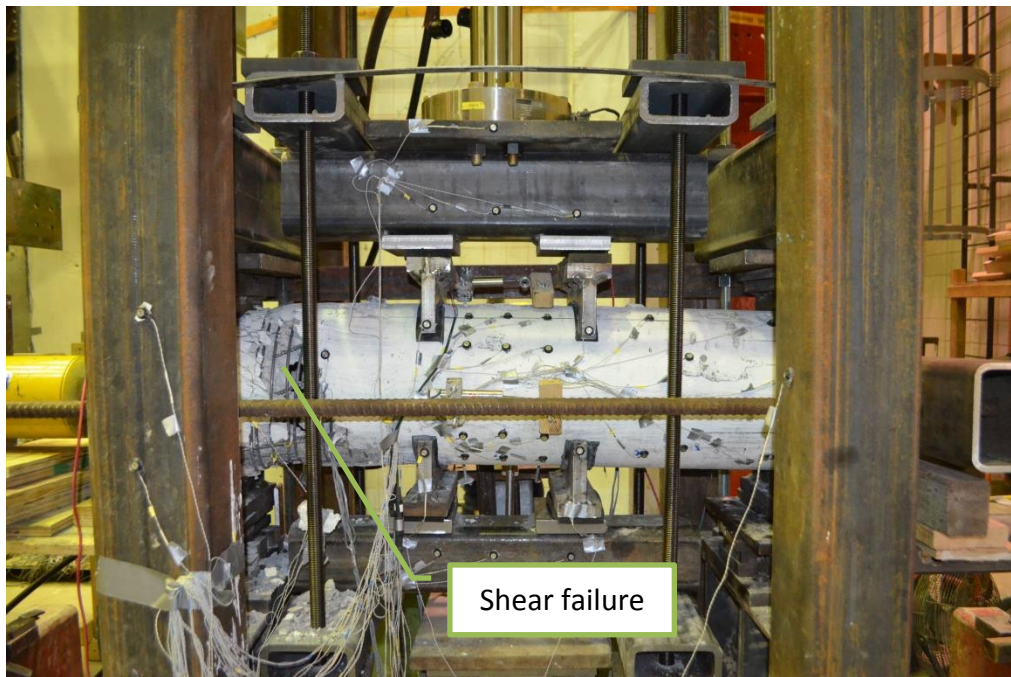
Figure 5-16: Specimen H1C2-C after Shear Failure
