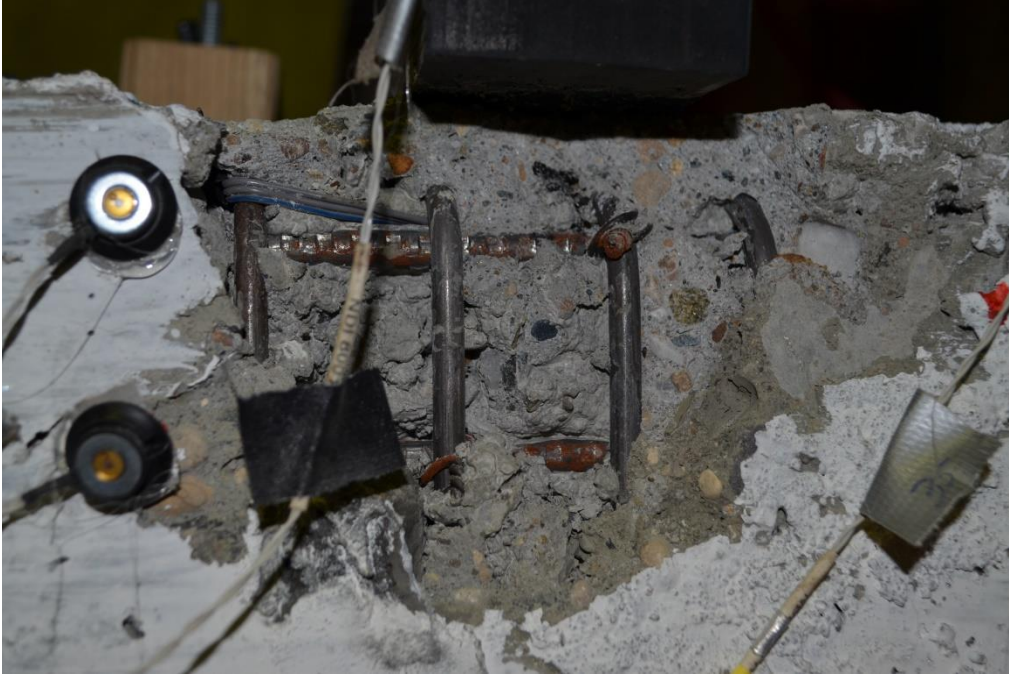
Figure 5-71: Specimen H2S3-C Close-Up of Local Cover Crushing at Load Point while Unloaded Prior to the Second Part of the Cycle at F_y
