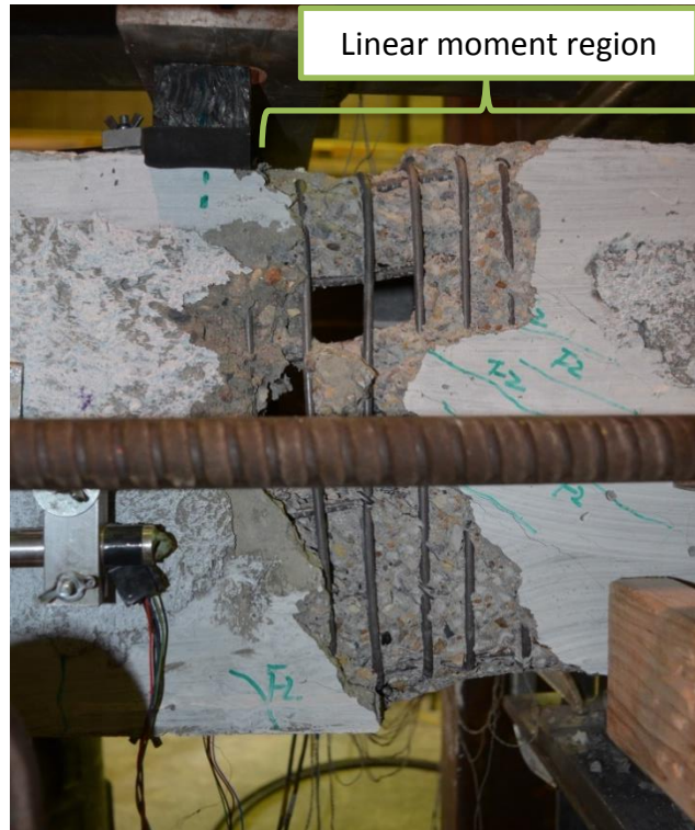
Figure 5-74: Specimen H1.25S1-M Shear Failure in the Linear Moment Region
